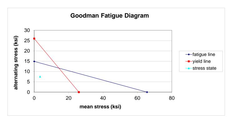
Conclusion: The Safety Factor falls just short of the recommended min. of 2. However, the Goodman Diagram shows the stress level well below both the yield and fatigue line for infinite life. The shaft is approved for use in this application.
