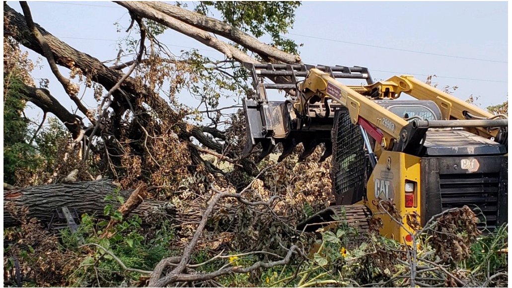
Above: A 299D3 with a grapple bucket cleans fallen trees in Springville, IA. The First Response Team of America (FRTA) used donated equipment from Altorfer Rents to clean up the community after Iowa's derecho on August 10.
