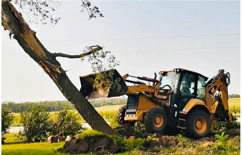
Above: A 420FL backhoe takes on a damaged tree in Springville, IA. First Response Team of America (FRTA) was in Iowa for five days clearing storm damage.
